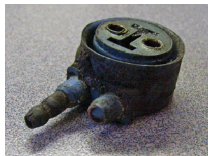
» A corroded lamp connector shows signs of environmental stress and systemic corrosion.
